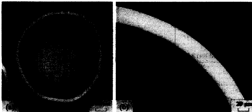
Fig. 1. Optical micrographs of polished cross-section of irradiated ZrC–Triso coated fuel particle before heating test.
